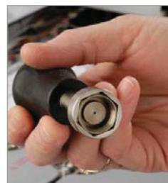
Septum nut remains in tool until reinstalled.
