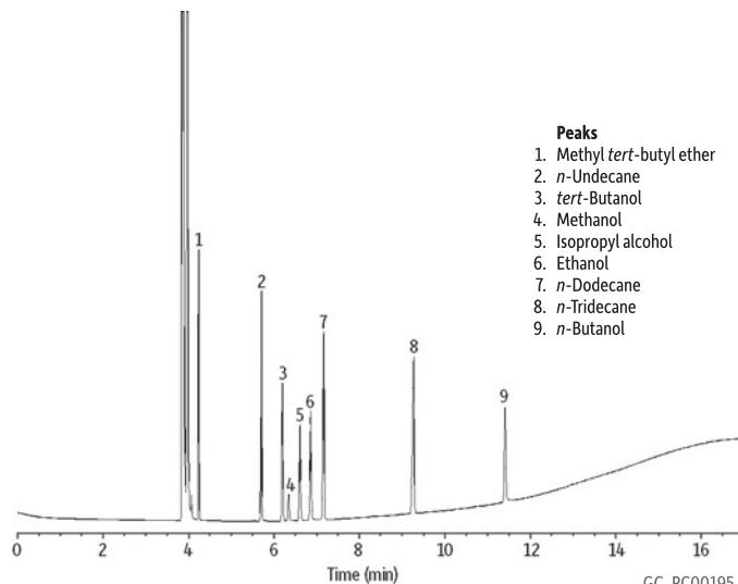
Column Sample: Rt<sup>®</sup>-TCEP, 60 m, 0.25 mm ID, 0.40 µm (cat.# 10999)
