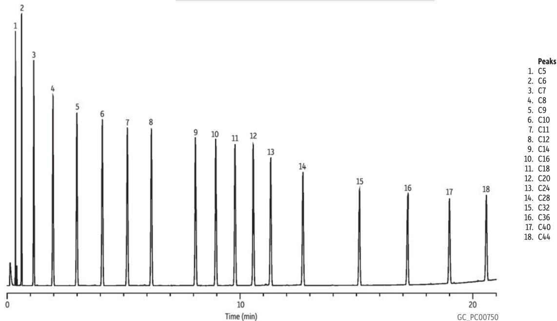
**Column** Rtx®-2887, 10 m, 0.53 mm ID, 2.65 µm (cat.# 10199)
