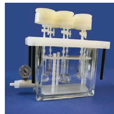
Fully assembled unit shown with glass vacuum chamber (cat.# 25991) and disk holders (cat.# 24020).
