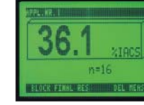
The simple display mode is available for applications where only the current display of the electrical conductivity and the number of performed measurements is of interest. The temperature compensation of the conductivity can be activated in this mode of operation as well
