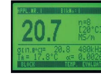
In the scientific display mode, the temperature taken by the sensor as well as the temperature coefficient used for the temperature compensation of the electrical conductivity are displayed in place of the mean value and the standard deviation. Additional instrument functions can be selected by using the softkeys in the lower LCD region
