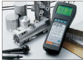
The electrical conductivity measurement is employed for the production, processing or inspection of finished goods (e.g., EURO coins) made of NF metals
