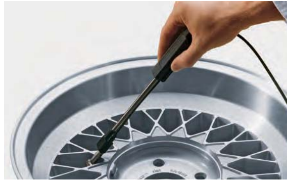
Measurement of the lacquer thickness on an aluminum rim wheel with the probe FAW3.3, mounted in the guiding device
