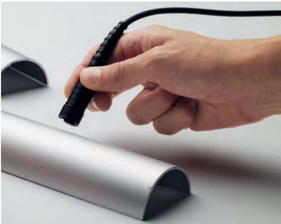
Measurements of anodized coatings with the curvature-compensating probe FTD3.3
