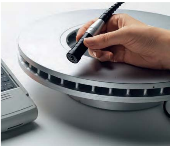
Measurement of zinc powder coating with the two-pole probe V7FKB4
