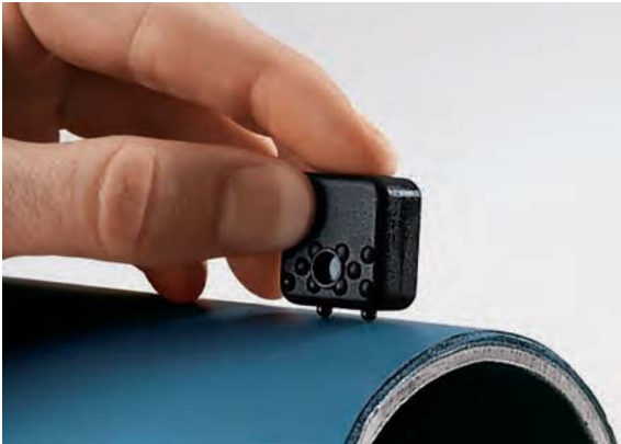
Measurement of the corrosion protection coating in plastics on steel pipes with the probe FKB10
