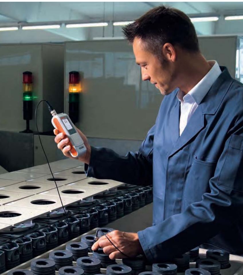
Quality monitoring on engine pistons after the manufacturing process using the FTA3.3H probe
