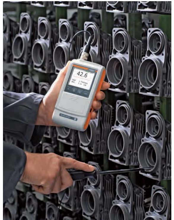
Measuring with the internal probe FAI3.3-150
