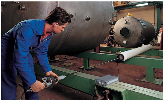
Testing of the interior coating of a pipe with a rotating electrode on a rod system and the POROSCOPE®
