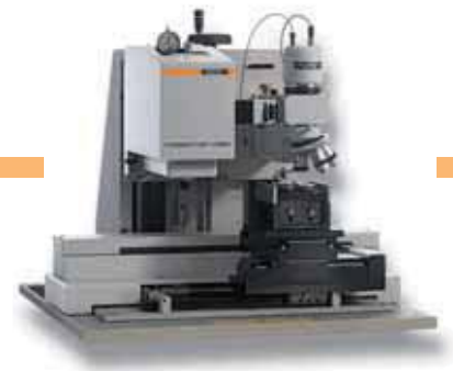
2004 FISCHERSCOPE® HM2000 and PICODENTOR® HM500: Wider load range (HM2000) and increased vibration stability for industrial applications
