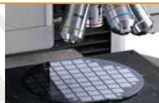
Automated measurements on a wafer
