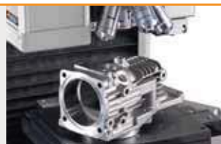
Microhardness determination on a gear housing
