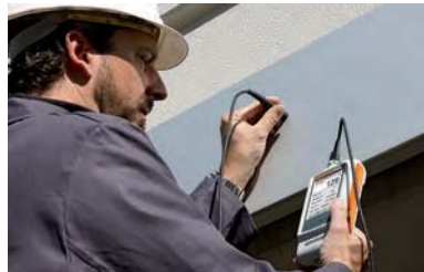
Measurements of anodised aluminum on a façade
