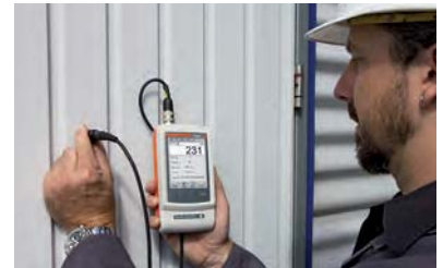
Measurement of paint coating thickness
