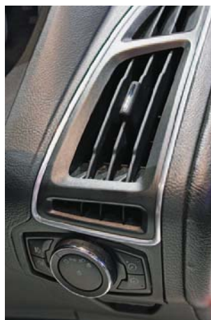
Typical application for the CMS2 STEP: chrome-plated trim elements in automotive manufacturing, based on multiplex nickel coatings
